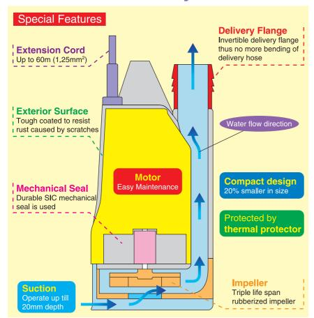
Triple life span due to special rubberized impeller as compared with cast iron impeller.
