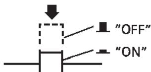
The DC circuit breaker turns off automatically when DC charging circuit is overloaded or the battery has problem.
