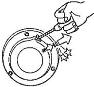
To start the engine, pull slowly on the recoil starter until it is engaged, then pull it briskly.
