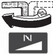
When starting a cold engine, turn the choke lever to CLOSE “|” position.
