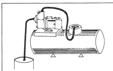
2. When installing the pump upon the fuel tank, install the pump above the tank. Installing the pump underneath the tank is not advisable due to natural flow of liquid by a siphon action.
