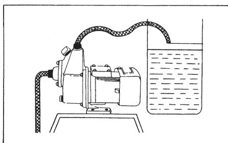
4. Be sure to raise the end of the delivery hose and delivery pipe from the level of the lifted liquid. Immersing the end of the hose or the pipe in the liquid will cause the liquid in the pump to be discharged by the siphon action so that the pump will fail to demonstrate the self priming action.
