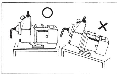
3. Install the pump horizontally. Being a self priming pump requiring the liquid to be invariably present in the pump, installing it aslant may cause the liquid in the pump to become insufficient and the pump may fail to demonstrate its self priming action.
