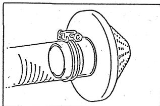
! CAUTION: Do not remove strainer or pump damage may occur by foreign material.
