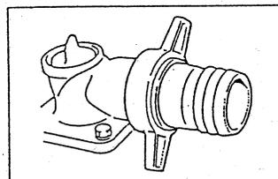
1. ○ Install the hose joints on the pump.
