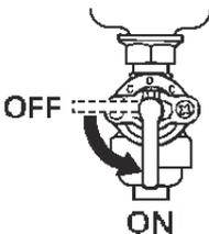
Before starting the engine, turn the fuel valve to "ON" position so the fuel flows from the fuel tank to the carburetor.
