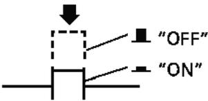
The DC circuit breaker turns off automatically when DC charging circuit is overloaded or the battery has problem.
