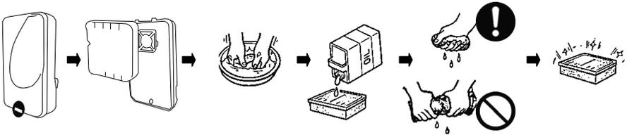
**CAUTION** The engine should never run without the element, excessive piston and cylinder wear may result.
