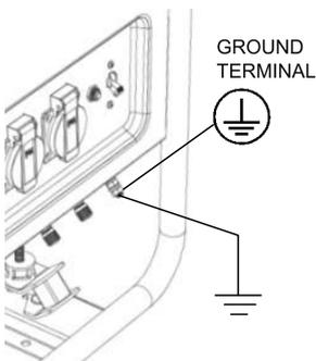
Make sure to ground the generator to prevent electrical shock. Connect the ground lead between the ground terminal and the ground.
