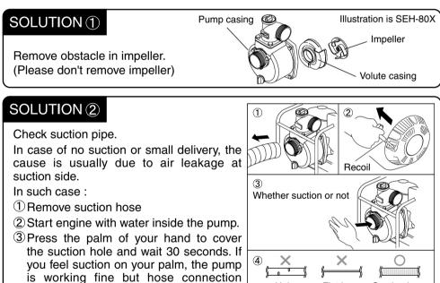
needs correction. ④ Please check if rubber packing is installed and if there is any hole on suction hose.
