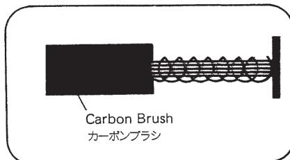
When ordering carbon brush, specify the model name of your machine, such as FS-3224S and FS-2024S.
